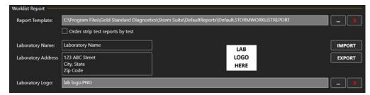
Laboratory name, address, and logo can be exported to an .xml file and later imported, if the same information should be used in multiple instrument systems, using the Import and Export buttons.
