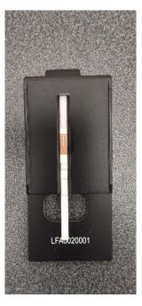
The cassette is then placed into the reader such that the numbered end of the cassette faces out of the reader, as shown in the images below.
