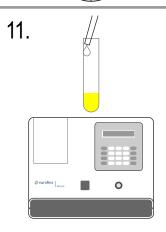
Add 500 iL of Stopping Solution down the inside wall of each tube by using the technique previously described. Read results at 450 nm within 15 minutes after adding the Stopping Solution. Multiply results of samples by the appropriate dilution factor (if any).
