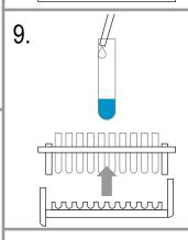
Lift the upper rack (with its tubes) off the magnetic base; add 500 ìL of Color Reagent down the inside wall of each tube by using the technique described in Box 2.
