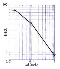
This test kit has a wide detection range between 0.02mg/L and 1mg/L.
