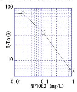
This test kit has a wide detection range between 0.02mg/L and 1mg/L.
