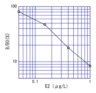
Samples containing E2 within the dynamic range between  $0.05\mu g/L$  and  $1\mu/L$ . can be directly applied to assay after filtration. E2 content below the range must be concentrated with solid phase extraction prior to the ensuing session.
